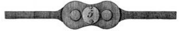
Plan of the Cross joint at every 10 th Link.
